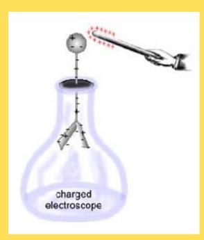
If a loaded body approaches the knob and touches it, then part of the charge will be transferred to the rod and then to the leaflets for contact charging
